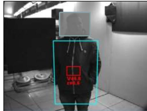
Data are processed in real time to estimate **volume** and **dielectric properties** of the detected object and determine if it is explosive or not. The system is fully automatic and thus **operator independent** so **no special skills are required**.
